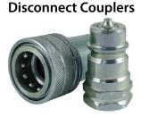
Recommended for general purpose, mobile hydraulics, machine tool, plastic molding and test equipment applications. Features Buna seals, double shut-off, and proven ball-lock mechanism for positive connection.
