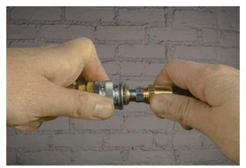
After pulling the sleeve, the plug will move out of the couple slightly. Continue to hold the hose and coupling sleeve until all air is fully exhausted.
