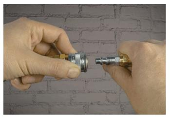
4 After the line is fully exhausted, you are able to safely separate the plug from the coupler.
