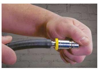
**2** Grip the Plug or socket firmly and Push On hose.
