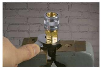
With even and smooth force applied, wrench tighten according to the "Turns From Finger Tight" values listed in the table below.
