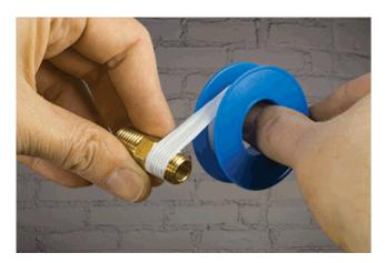
1 Apply 1-1/2 to 2 wraps of PTFE tape, starting one or two threads from the lead edge, in a clockwise direction. For type 316 stainless steel, be sure to use stainless grade tape.
