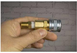
2 Check threads to make sure there is no damage and that tape is properly installed. Align threaded connections and carefully begin threading the two halves together.
